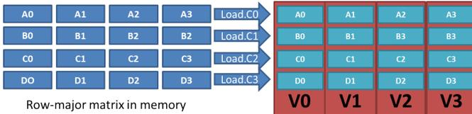
Fig. 3: Load-scatter to a quadruple register operand.
