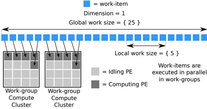
Fig. 6: OpenCL NDRange execution using SPMD Mode.
