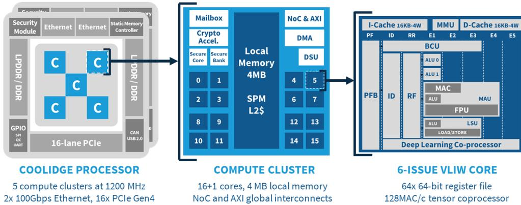
Fig. 1: Overview of the MPPA3 manycore processor.
